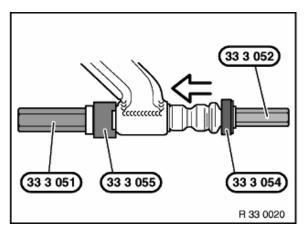
Coat new rubber mount with Circolight (refer to BMW Parts Service) and pull in with special tools 33 3 051/052/054/055.
